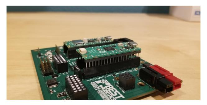
Slowly push the module downward (straight) from each end a little at a time until the pins slide in. When seated completely, there should be no pins visible.
