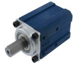
AndyMark 775 Motor and 57 Sport Gearbox ● 36:1 Gear Ratio ● 25.2 Nm Stall Torque
