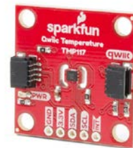
SparkFun Digital Temperature Sensor - TMP117 (Qwiic)
